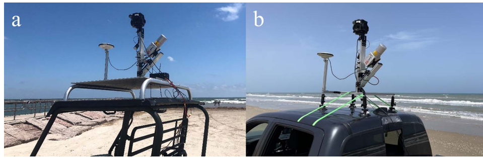
Figure 2. HiWay Mapper mapping-grade MLS system mounted on (a) a custom metal plate fitted over the roof of a UTV and (b) suction cups on the roof of a 4WD vehicle.
