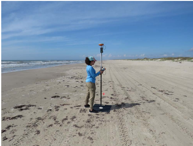
Figure 18. Visualization of Malaquite beach and example of target type and GCP placement.
